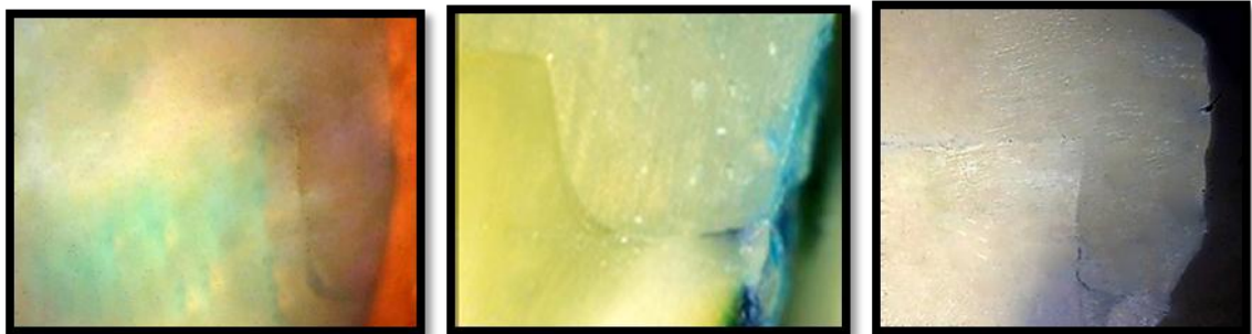
Figure 1: a) Dye penetration of samples of Group A (SR Nexco)
