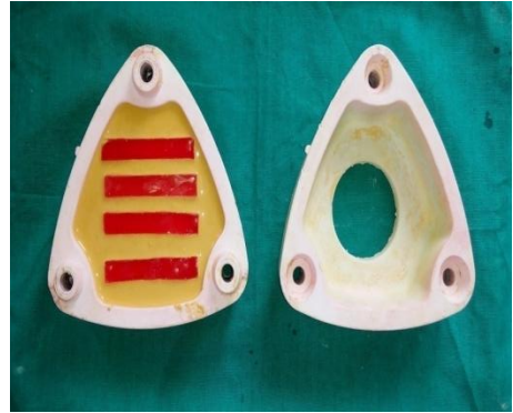
Figure 6: Flasking of microwave samples in ceramic flasks
