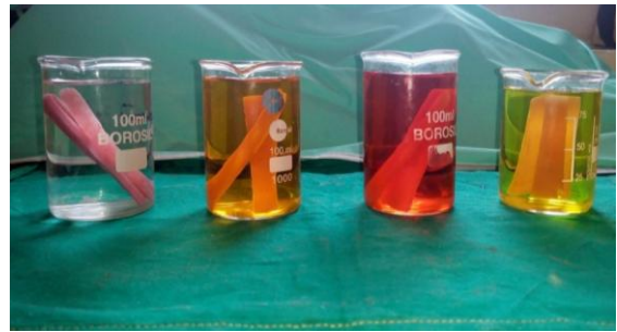
Figure 8: Acrylic samples placed in different coloring solutions
