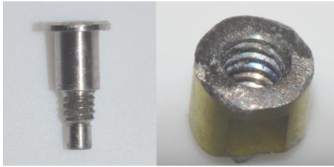
Fig.6: a) Male portion (cover screw) b) Female portion (threading)
