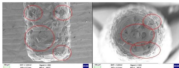
Figure 4: SEM image of Group B test specimen after tenth cutting cycle
