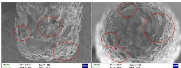
Figure 2: SEM image of Group A test specimen after tenth cutting cycle
