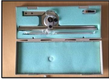
Fig 1: Bevel protractor for Buccolingual measurement
