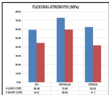
**Figure 3:** Mean Flexural Strengths (MPa) values of test materials after Long Curing Cycle and Short Curing Cycle
