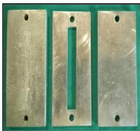
**Figure 1:** Customized 3 piece Aluminium mould
