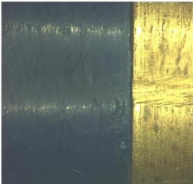
Figure 2: Measurement of marginal gap of wax pattern using optical stereomicroscope
