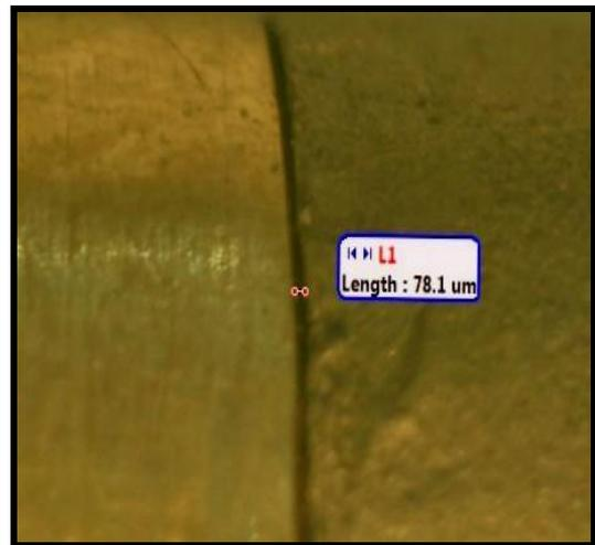
Figure 5: Measurement of marginal gap of casting using optical stereomicroscope.
