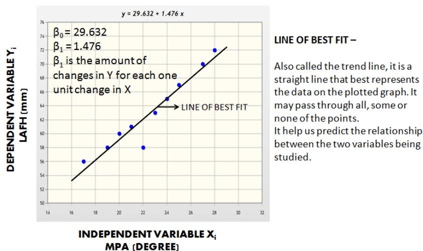
Figure III – Explaining the graph of the regression line.
