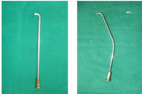
Figure 4: Straight And Bent Motorcycle Spoke
