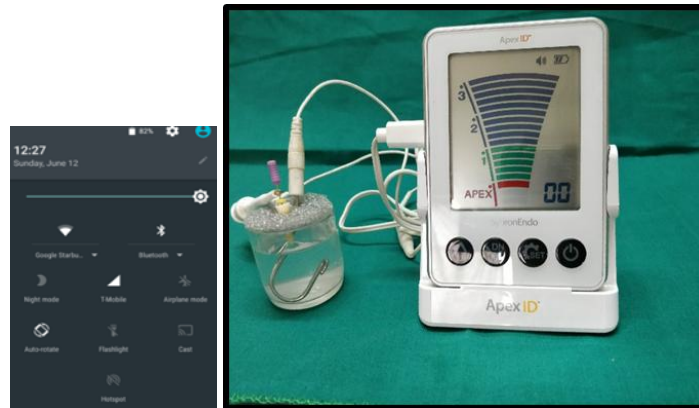
Figure 3: Group III - Apex ID at distance of 40 cm to 3G smart phone when Bluetooth and Wi-Fi is activated
