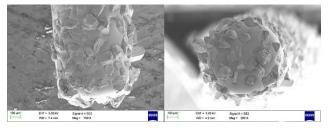
Figure 3: SEM image of Group B test specimen before initiation of cutting cycle
