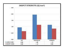
Figure 4: Mean Impact Strengths (KJ/mm<sup>2</sup>) values of test materials after Long Curing Cycle and Short Curing Cycle
