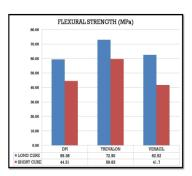
Figure 3: Mean Flexural Strengths (MPa) values of test materials after Long Curing Cycle and Short Curing Cycle
