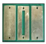
Figure 1: Customized 3 piece Aluminium mould
